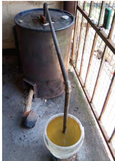
Fig. 4 – Batch reactor heated on burning wood (Owusu et al. , 2018)
